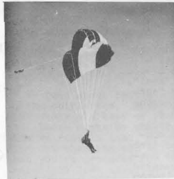
Ed Grimm (C-34), enjoying a soaring descent under the Wing. Note steering system on the trailing edge of the canopy.
